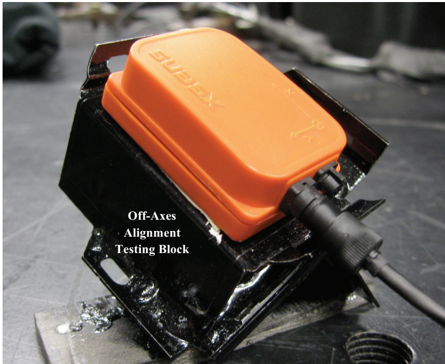
Figure 2. Testing block for dynamic vibration tests where all three sensor axes were rotated off-alignment from the global coordinate system. The testing block was rigidly attached to the motion shaker platform.
