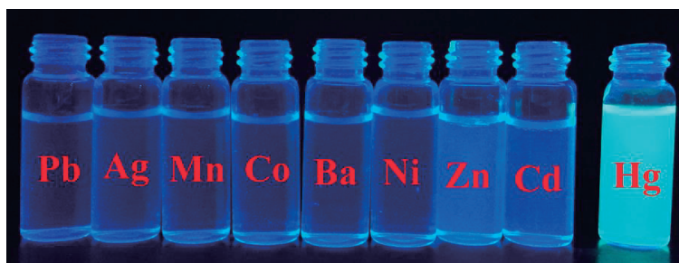
Figure 2. Digital photographs of compound 1 ( 5 \times 10^{-5} \text{ mol} \cdot \text{L}^{-1} ) upon addition of different metal ions (4 equiv) in DMF-water (5:95) mixtures solvent with a UV lamp ( \lambda_{\text{ex}} = 365 \text{ nm} )
