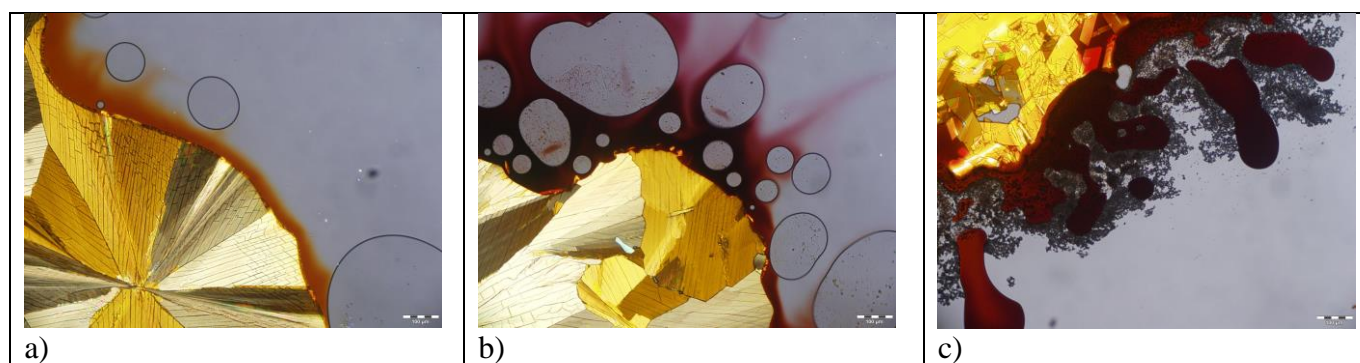
Figure 1. Polarized light photomicrographs of the recrystallized melt of the yellowish colored, dichroic 2-(4-fluorophenyl)diazenyl)-1,3-diethylimidazolium tetrafluoroborate ( 5 ) in contact with the undercooled melt of (a, b) tetrabutylammonium azide (Mp 89 °C) and the melt of (c) KSCN (Mp 175 °C). a) image recorded at 70 °C (start of the reaction); b) at 80 °C showing the fast production of nitrogen bubbles under formation of a deep purple secondary dye diffusing into liquid Bu_4N^+N_3^- ; c) contact zone after melting KSCN at 175 °C resulting in a deep purple dye and a greyish precipitate (supposedly KBF_4 ).
